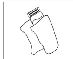
1. Add more than 10ml of the solution to be tested, tighten the bottle cap, and add carefully to avoid air bubbles.
