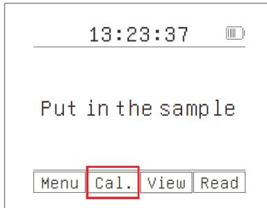
1. Click "Calibration" on the main screen to enter the "Confirm Calibrate" screen.
